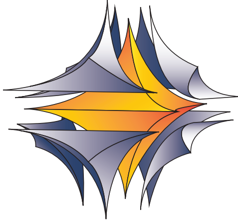
FIGURE 8. The maximal volume generalized octahedron decomposes into one ideal regular octahedron and eight tetrahedra that recombine around their finite vertices into a single additional ideal regular octahedron.
